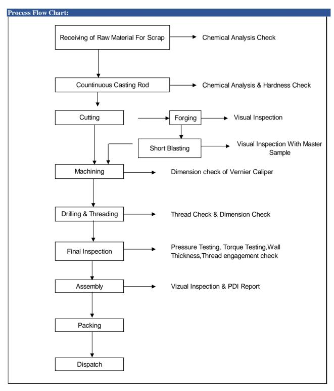
This flow chart visually represents the sequential steps involved in the production process of extruded brass rods and forging parts, starting from raw material collection and sorting, through various processing stages, quality control, and ending with packaging and dispatch of the final products. Detailed Breakdown of the Process for Converting Brass, Copper, and Zinc Scrap into Extruded Brass Rods and Forging Parts:
